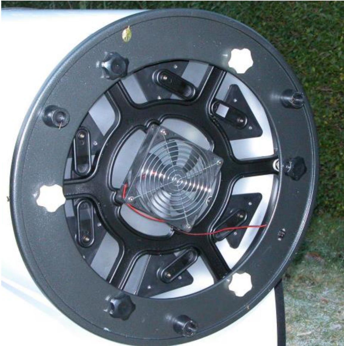
Photo 5: Rear view of mirror cell with collimation mechanism and cooling fan
