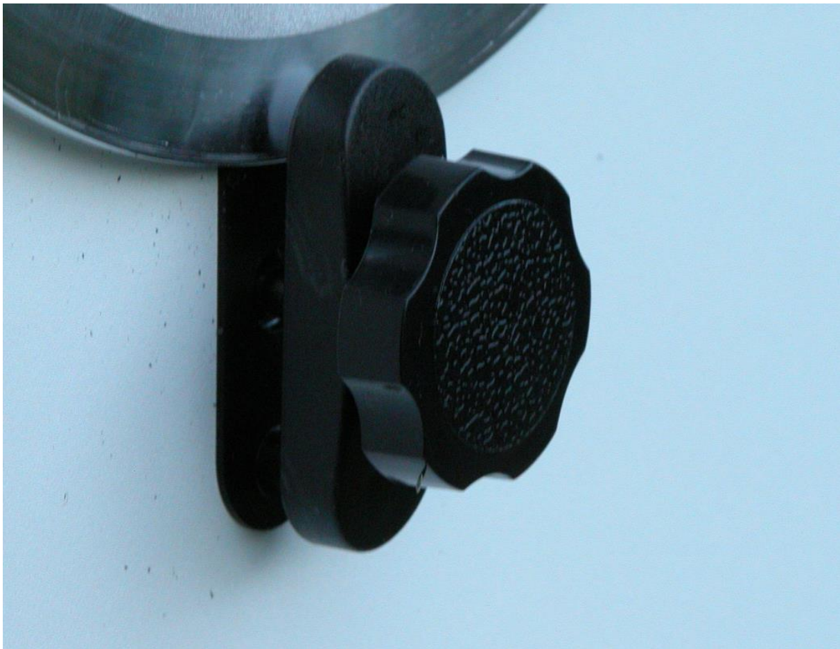
Photo 2: friction mechanism for balance control
